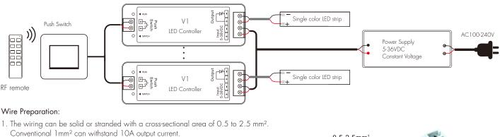
2. When wiring is installed, the terminals must be tightened. If they are not tightened, the contact point resistance will be too high and the terminals will easily burn due to heat when used at full load for a long time. 0.5-2.5mm<sup>2</sup>
